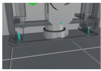
If uneven floors (eg. slope towards the drain) cistern can be adjusted using the adjustment screws found on the bottom of each side. 5970-MA can be adjusted from above with a hexagon wrench, M5. 5970S3-EL can be adjusted from above by hand.
